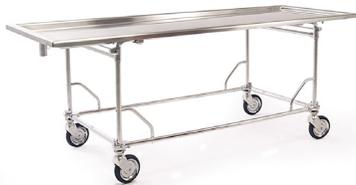
The Model 103 Combination Operating Table is a multipurpose table, ideal for embalming, transferring and dressing. For added convenience, each end can be adjusted independently for individual working height and drainage. The stainless steel top is durable and rigid, featuring a convex surface and deep side troughs for efficient drainage without the need for splash guards. It features 6" wheels with lock to keep table stationary while in use.
