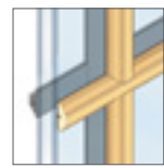
Simulated-Divided-Light without Spacer 7/8"
