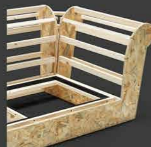
• Frame With Osb - Plywood & Fir
