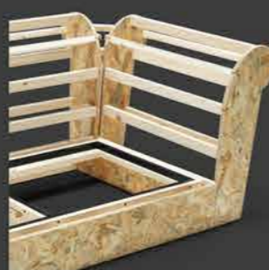
• Frame With Osb - Plywood & Fir
