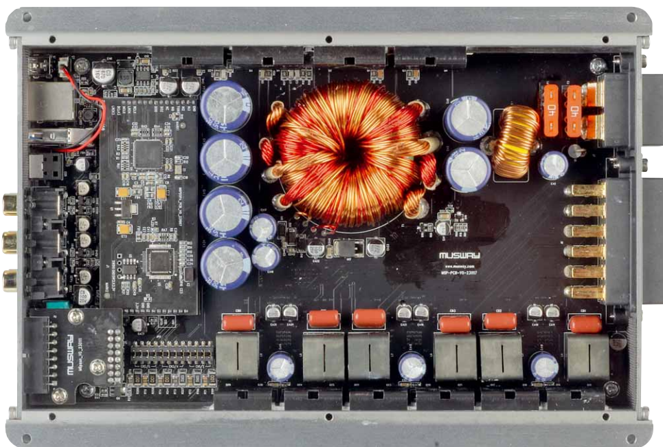
The massive transformer power supply supplies 6 identical channels that are fired via MOSFETS
