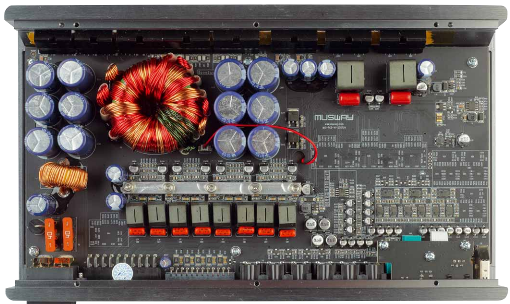
The 8 small channels are located under the powerful power supply with an XXL transformer. the larger coils belong to the top right the major canals
