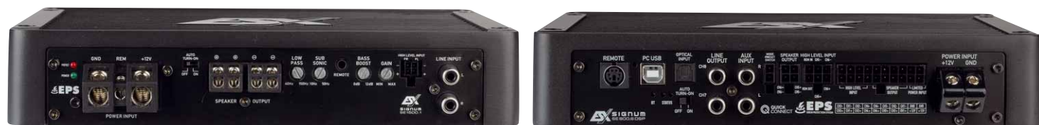
On the left the 1500.1 with strong terminals and double connectors for thick wires, on the right the 800.6 with Molex multi-pin connectors for the 6 inputs and outputs
