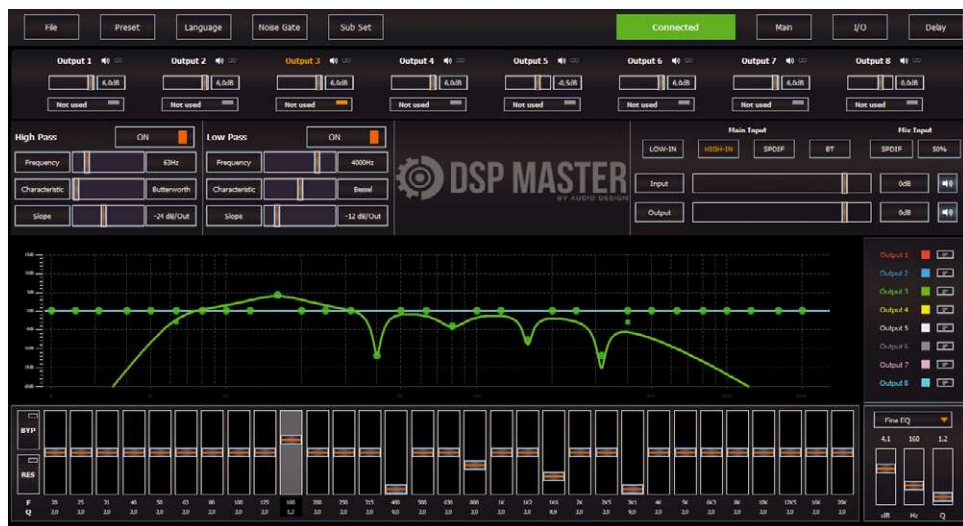
In the main window there are levels, crossovers and 31 EQ bands for the channels
