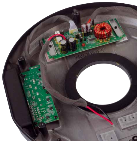
Above the power amplifier board with a classic Class-AB circuit and transformer power supply
