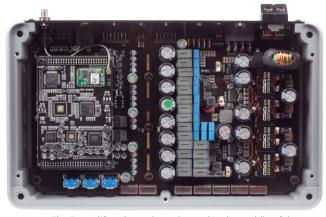
The 7 amplifier channels are located in the middle of the very high-quality multi-layer board, below are the amplifier ICs
