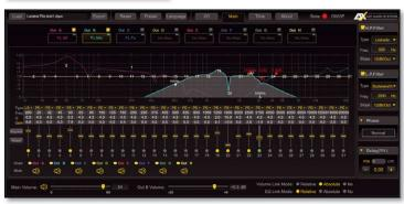
Equalizers and crossovers are set in the main screen. Master and channel levels are available and absolute or relative linking of channels is possible
