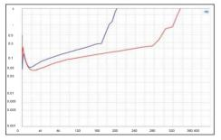
The VX1400.4 PRO offers performance to the max. With over 180 watts at 4 ohms and over 320 watts at 2 ohms, it is one of the performance monsters. On the other hand, the distortion of 0.05  $\cdot$  0.3% is not record-breakingly low for a four-channel power amplifier
