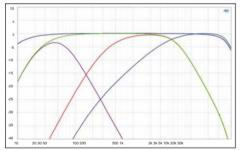
The VX1400.4 PRO runs up to 40 kHz and offers frequency crossovers up to 5 kHz, with the high-pass filter of the front channels changing the edge steepness somewhat sloppily
