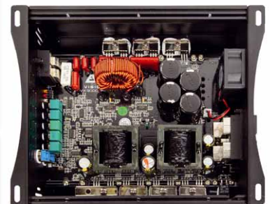
In contrast to the VX2000 PRO (above), the VX3000 Pro has two mains transformers
