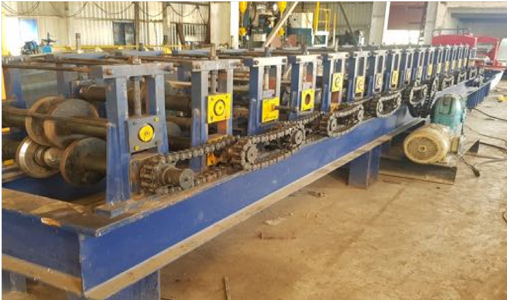
"C" Purlin machine 350mm x 3mm Capacity
