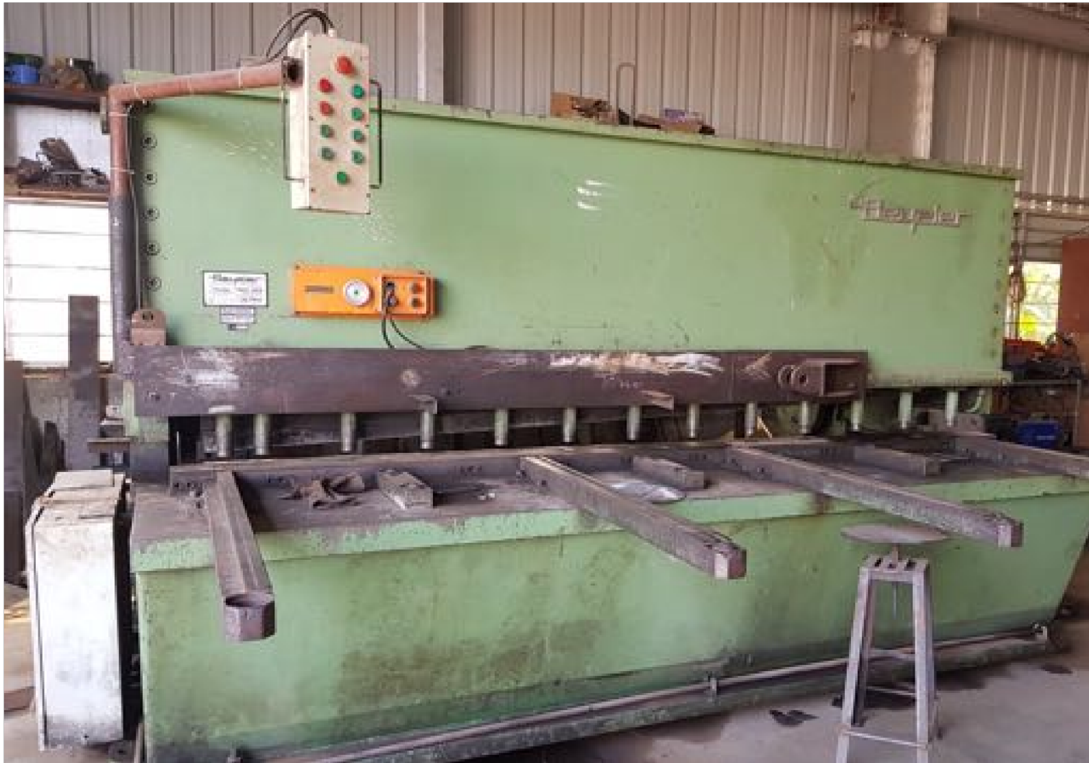
20 mm x 4,000 mm Capacity Shearing machine
