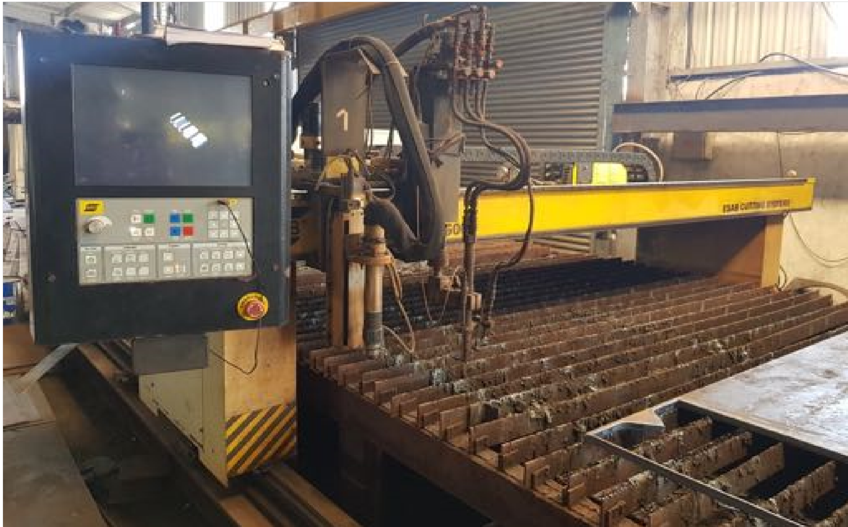
3M X 13M PLASMA & OXY FUEL CUTTING MACHINE (Plasma capacity = 40mm)
