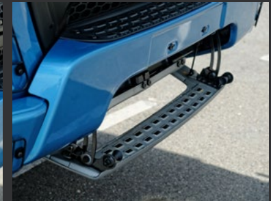
Folding anti-slip platform for better windscreen accessibility.
