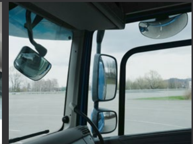
Extra mirrors provide a clear view of the truck's surroundings.
