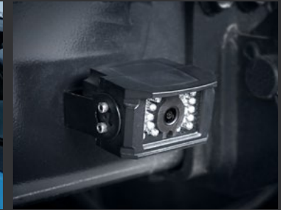
Reversing camera for a better view of what's happening behind the vehicle
