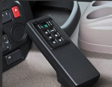
Automatic transmission control.
