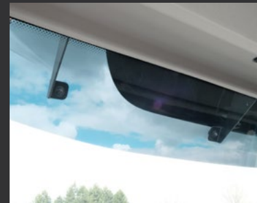
Sun visor reducing sunlight penetration and preventing the cab from overheating.
