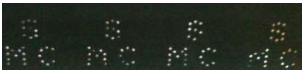
Figure 4 – Punching on black cardboard shows the four die strikes
