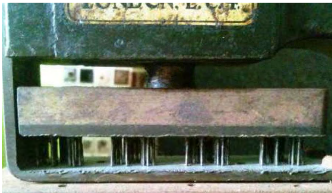
Fig. 3 – Close-up platen showing the pins.
