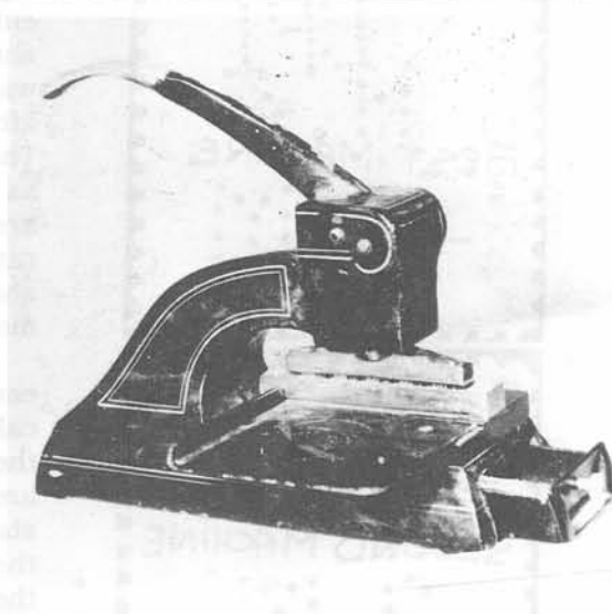
Figure 1. The Department of Finance used their Cummins Model 52 perforator to perforate the five-hole OHMS pattern. The machine could perforate five small stamps across and three stamps deep.
