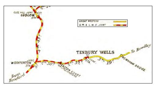
The above diagram (dated 1929) is from a book of Junction Diagrams produced by the Railway Clearing House. It clearly shows the Great Western Railway and the London Midland & Scottish Railway having joint running powers from Tenbury Wells to Woofferton Junction, where it connects to the jointly run Hereford-Shrewsbury main line.
