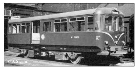
As well as specialist sports cars (such as the AC Cobra), the company also built four trains for the Southend Pier Railway (in 1949), and five 'Railcars' for British Railways - W79975/6/7/8 and SC79979. As the Thames Ditton works had no rail connection, and the works doors were too small, each 'Railbus' left the factory by road in two parts, then assembled off-site. Introduced in 1958, they were all withdrawn by 1968, no doubt killed off by Dr Beeching's cuts.
