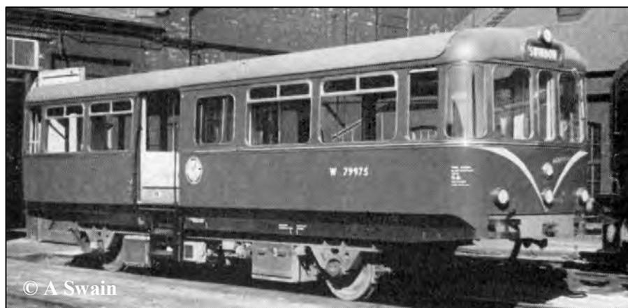
As well as specialist sports cars (such as the AC Cobra), the company also built four trains for the Southend Pier Railway (in 1949), and five 'Railcars' for British Railways - W79975/6/7/8 and SC79979. As the Thames Ditton works had no rail connection, and the works doors were too small, each 'Railbus' left the factory by road in two parts, then assembled off-site. Introduced in 1958, they were all withdrawn by 1968, no doubt killed off by Dr Beeching's cuts.
