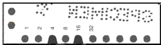
Fig 3. Sample coding with a binary number series added to the card in Fig. 1 to give a 'state' field.
