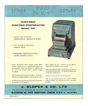
The Model 60 provided instant automatic perforation and of documents. As the paper was inserted it made contact with a microswitch. which in turn activated a motor to power the perforating mechanism. There was also an auxiliary option using a finger trip button. The sales features stated that no pedal or lever was necessary to actuate the process, thus eliminating operator fatigue with the use of a single Additionally, it provided hand. increased productivity and being
