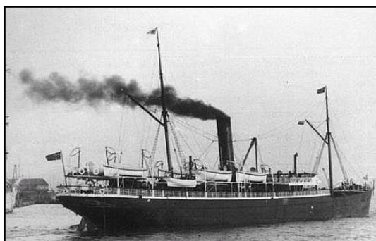
The s/s **ROMEO** built by "Earle's Shipbuilding & Engineering Co Ltd" in 1881 for the "Wilson Line" - 1,885 tons, with a service top speed of 12.5 knots.
