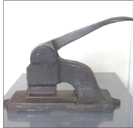
Single headed machine for producing advertising label JS/Co
