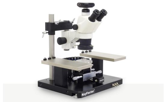
**Superscope** – Superscope has a turret for 4 M Plan APO lens. The magnification range could be 20X~2000X with 2X~100X objectives. This system is generally set up for probing on tiny geometric structures of wafer level reliability tests, failure analysis, high power tests, etc. InitialPS' intuitive manipulation enables users focus more on their measurements rather than manipulation.
