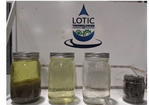
1-First pass sample, unfiltered; 2- First pass, filtered; 3- Second pass, filtered, 4- Second pass solids removed from over 60 L of water.
