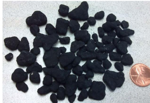
Figure 1. Configuration of PAC-coated particle.
