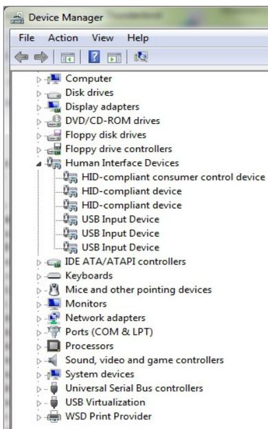
As of 8/9/2011 Aberlink now uses the white Fortress Keylok. This uses the standard built-in Win7 and WinXP, HID drivers, so no separate driver is required. Functionality is the same as the old green Keyloks.
