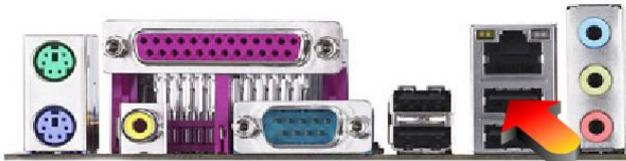
White keyloks can use any USB port, traditionally green Keyloks and Dongles have used the USB port below the Network port, as shown left.
