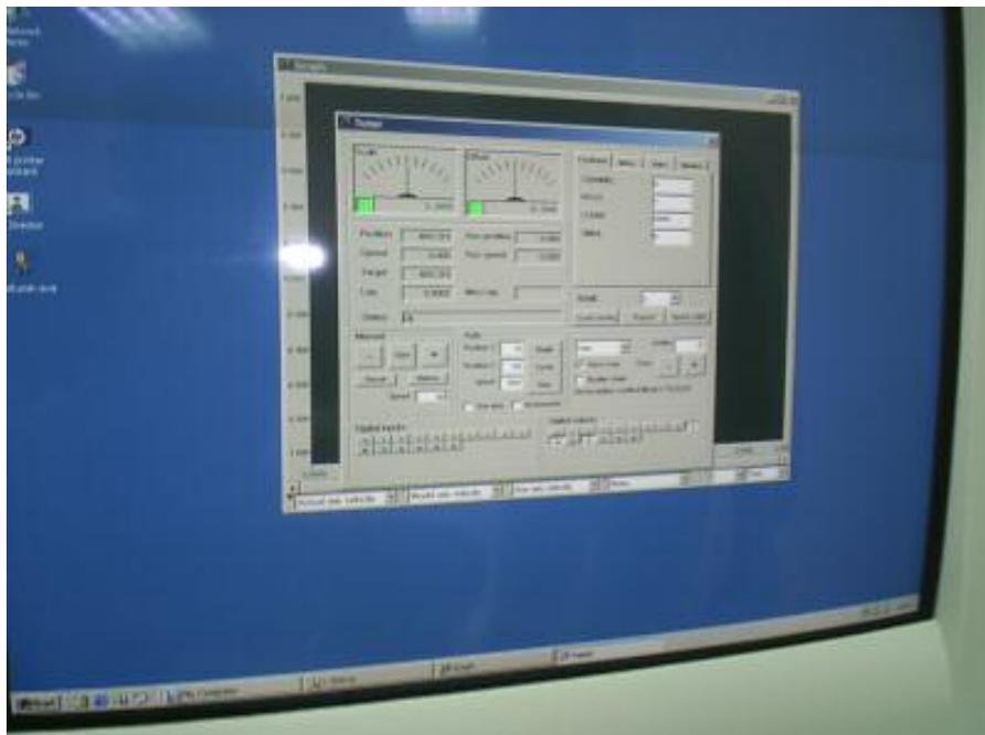
With axis tuner you can turn the amp on or off and turn the air on and off.
