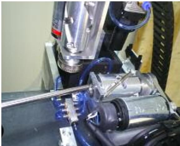
Repeat procedure for the X axis, push the carriage to the endstop then tighten screw, to avoid misalignment between rail and x axis.
