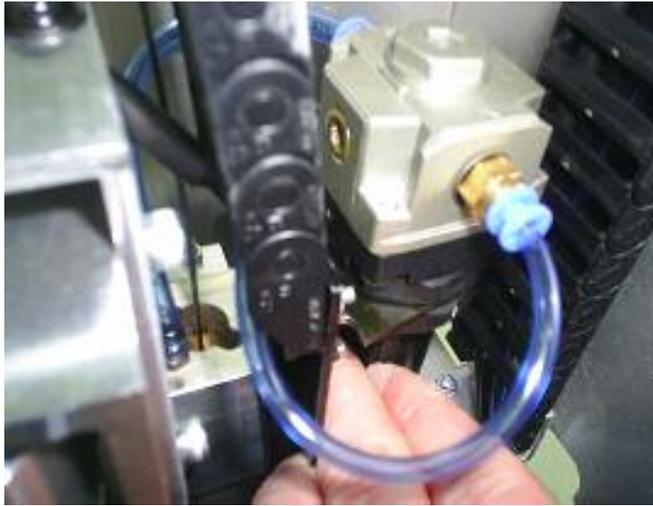
Open z balance regulator fully, this is in preparation for setting the balancing pressure – **note**, with this fully open the balance will not take the weight, and the z will drop when air is switched on, so make sure z axis is resting on the endstop, or something is under the bottom of the z quill.
