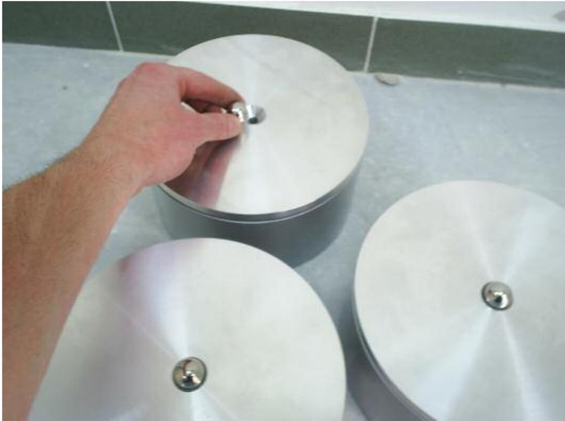
Position the feet as close as possible to where the machine will be located.
