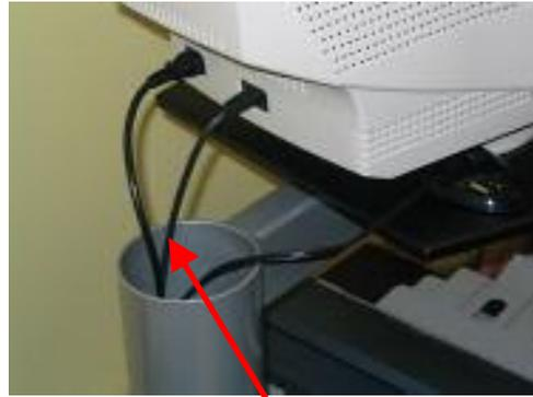
Connect dongle into free USB port, **s/w will not without it** and feed monitor cables and mouse receiver cables as shown
