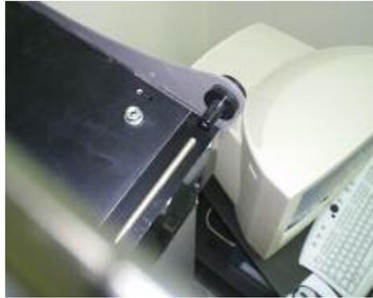
When securing the end nearest the ref. mark move the bridge all the way to the end, to make sure the end stop locates o.k in the hole in the bridge.
