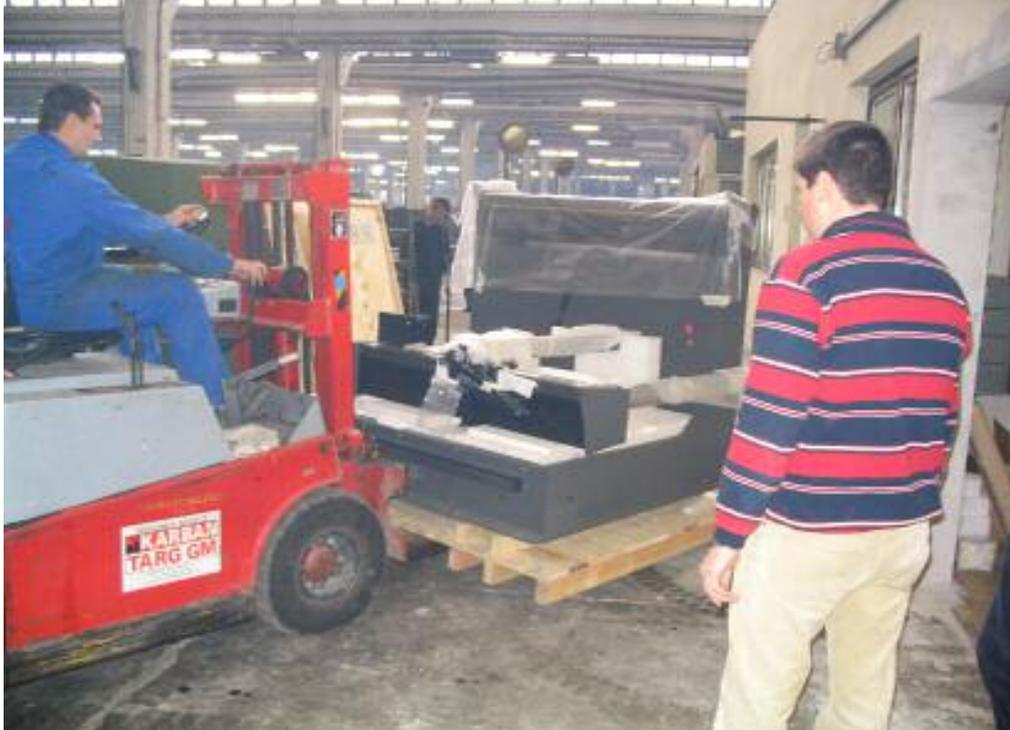
Slowly lower the machine and move the feet so the ball locates correctly. Before the granite can be moved into position the bridge must be moved to the side of the machine, so the granite has no obstruction. The photo below shows the bridge placed on a trolley beside the machine to allow clear access to the granite.
