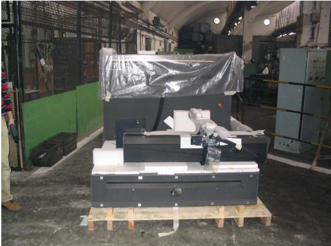
Next remove the three long bolts from under the crate base the bolts are 160mm long M10 with 17mm A/F nuts. Two are located at the back the third is at the front.
