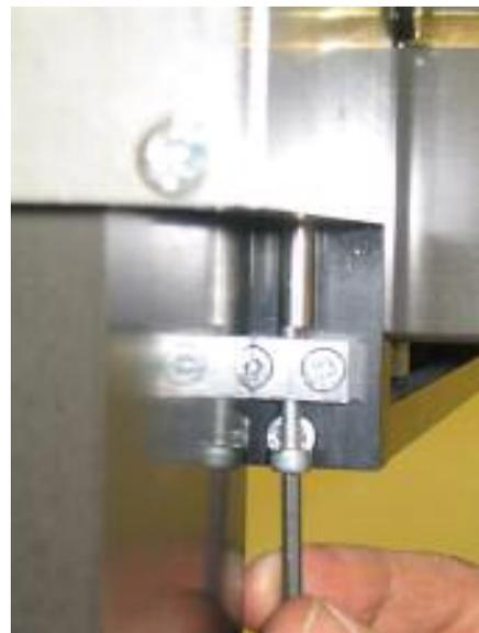
Position the bridge so it is at the front of the machine to give enough room for the rail. Locate the drive rail, which will not have the black end stops, the bar has a internal thread at one end. Push it up from the bottom of the carriage and push it through the bore of the drive drum, push until it locates in the rubber boot at the top of the Z cover, and secure rail by using the screw as shown in above picture.
