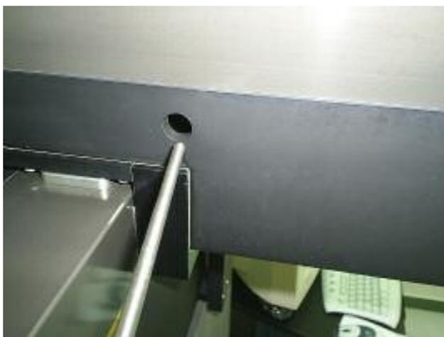
Locate the Y axis drive rail, which is the longer of the two, one end of the rail has the black end clamp fixed to the rail. The fixed endstop needs to go at far end of y axis, nearest the ref. mark
