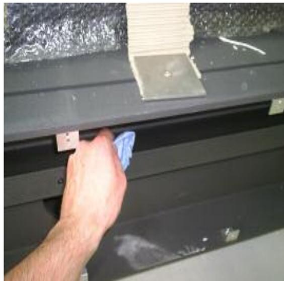
Also clean all air bearings on the bridge where the bridge mates with the chassis.
