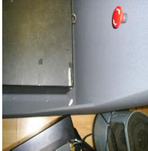
Position granite so it is 80-90mm from the back of the machine and 80-90mm from the front of the machine, ensuring granite is square to the machine, then remove straps and eye bolts.
