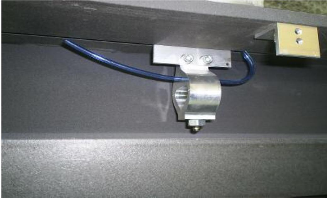
Locate the airbearing on the ball ended stud, and feed air pipe as shown, this bearing may also be feed from the narrow end, the bearing rotation is restricted by a pin in the pear drop which locates in airbearing (not shown above)
