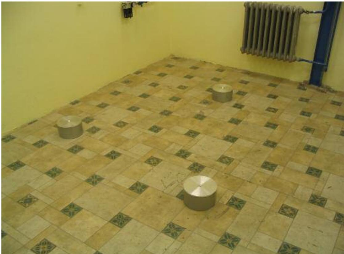
Next, using suitable lifting equipment, ideally a fork lift, lift the zenith machine from underneath and remove the base of the crate, next move machine to its position which should align with the three feet already positioned. The balls in the feet must locate with the mating part under the machine, if you look under the machine you should clearly see where the balls locate.
