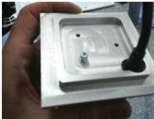
Feed probe cable through the probe plate and secure probe via the 3 screws – Make sure screws are tight and obviously line up front of probe with front of machine.
