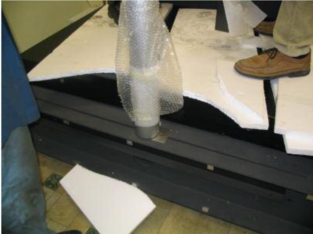
Using at least 3 people lift the bridge into place, in order for the left leg bearing holder to fit through the slot lift the bridge several inches higher and lower the bridge squarely downwards, one person needs to guide the left leg. Also position the metal plate (used in the packaging) to hold the left leg slightly off the chassis.
