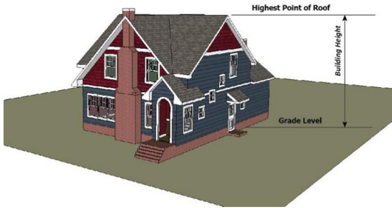
Figure 8-K: Measurement of Building or Structure Height
