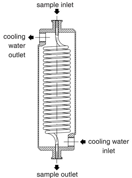
**Sample connection:** (inlet/outlet) 1/2" Tri-Clamp®
