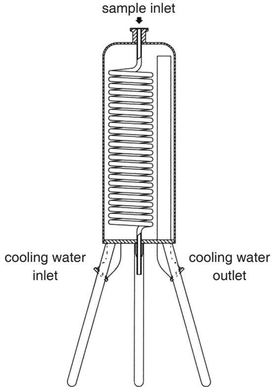
Sample inlet/outlet connection: 1/2" Tri-Clamp®
