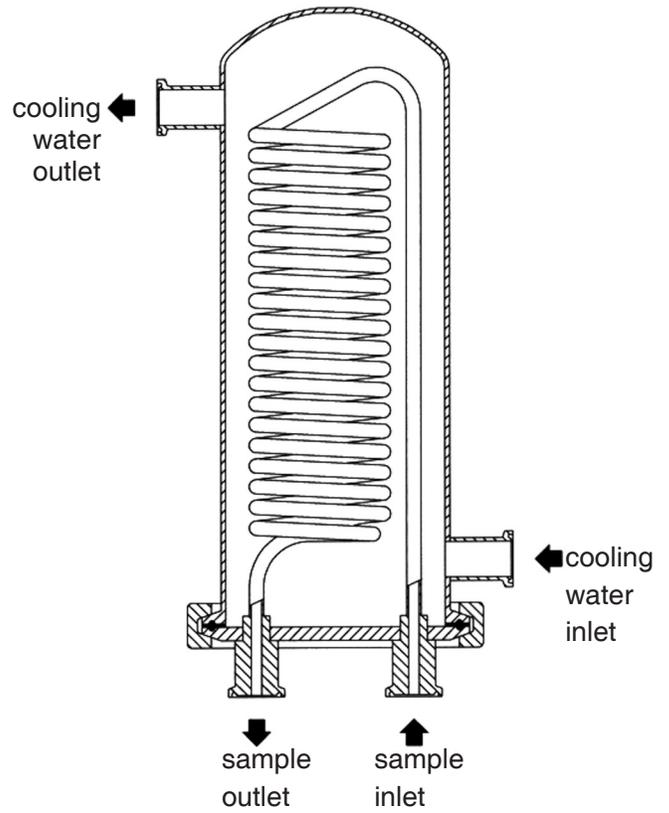
Sample connection: (inlet/outlet) 1/2" Tri-Clamp® compatible
