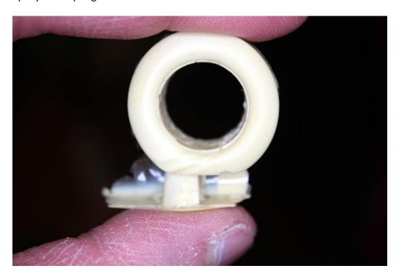
The finished tire – cast and ready for clean-up and use.
