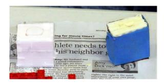
To the left are the two types of molds. The white block is the aircraft nose cone with a part in the mold that was poured from what is shown as the top side of the mold. The mold to the right with blue masking tape is the tire mold and shows how a multi-piece mold must be taped to hold together and aligned for a good part reproduction.
