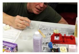
minute]. Vent holes are used for complex shaped parts so that the air in the mold can be pushed out as the resin is poured in. In some cases bubbles will appear on top of the pour surface and Ken will pop those before the material hardens. Bubbles will leave depressions in the casted parts surface. Those depressions can be filled with super glue during part preparation to remove them. For casting no release agent is needed.
