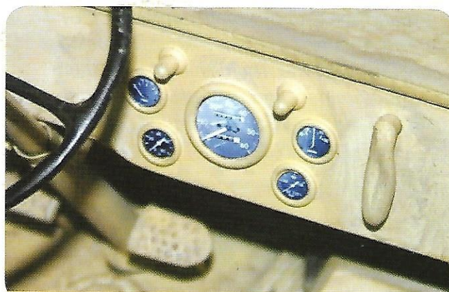
The original gauges were ground flat. I printed images of accurate instrument gauges on glossy photo paper to show the glazing.
