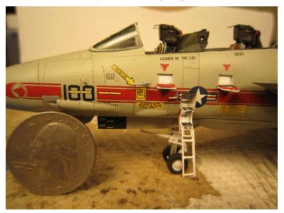
The completed cockpit tub was attached to the front wheel bay and this assembly was sealed between the forward fuselage sides, along with a hefty clump of lead weights. The forward landing gear is thin and not well supported, so it might be possible to put too much weight in the nose, and over stress the landing gear.
