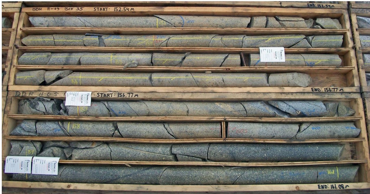
Drill core from DDH10-05:152.54– 156.77 m. Part of interval 8.80 m – 227.50 m averaging 604.7 ppm Cu, 42.4 ppb Au and 42.7 ppm Mo.
