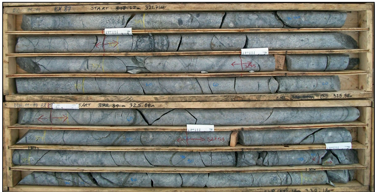
Drill core from DDH10-014: 321.71 – 330.18 m. Part of interval 207.5 m – 330.18 m averaging 54.52 ppm Mo (negligible Cu and Au).
