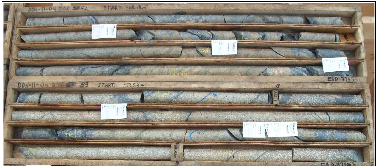
Drill core from DDH10-04: 368.18 – 376.95 m. Part of interval 319.00 m – 403.86 m averaging 356.7 ppm Cu, 9.6 ppb Au and 22.1 ppm Mo.
