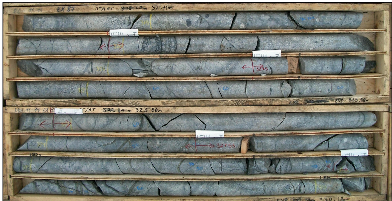
Drill core from DDH10-014: 207.50 – 330.17 m. Part of interval 207.5 m – 330.17 m averaging 54.52 ppm Mo (negligible Cu and Au).
