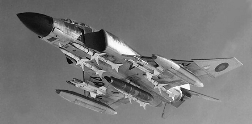
A Phantom FGR2 armed with four AIM-7E Sparrows and four AIM-9G Sidewinders plus a SUU-23 gun pod.
