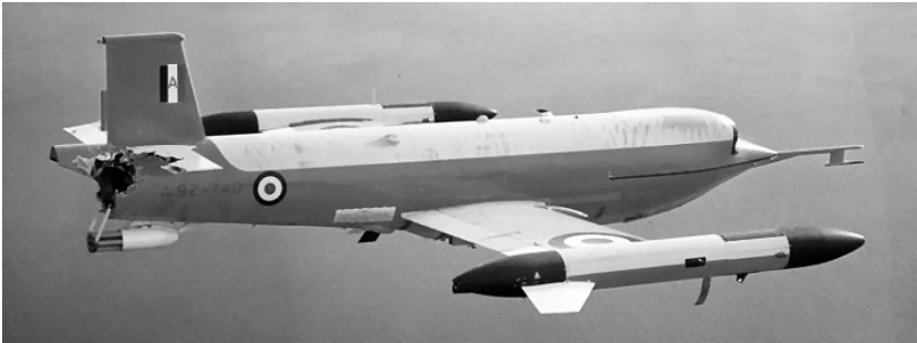
A Jindivik following an engagement with a Sidewinder training round that had ignored the towed flare and gone for the jet pipe instead.
