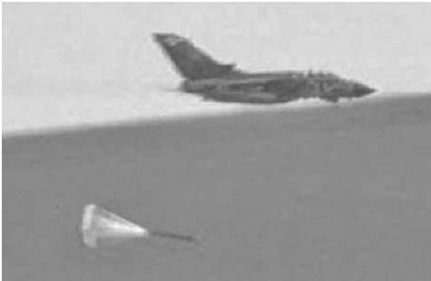
Trial release of a retarded WE177 from a Tornado.
