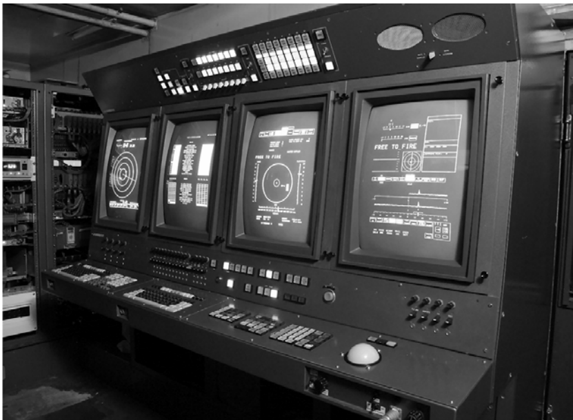
The LCPs were upgraded in the 1980s with introduction of the Argus 700 computer and a display suite with four 20 inch monitors.
