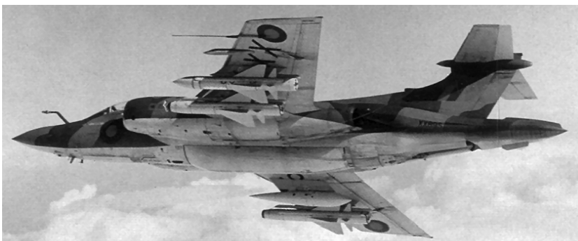
A Buccaneer with an anti-radar MARTEL (nearest) and a TV MARTEL under its port wing and, to starboard, the digital link pod and a second TV MARTEL
