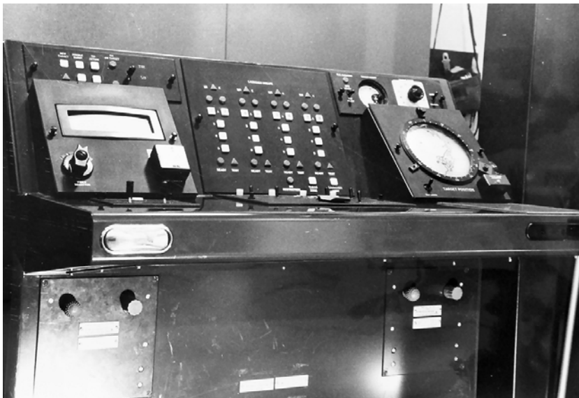
The missile operator's console within a Bloodhound Mark 1 Launch Control Post permitted him to control eight missiles and a TIR.
