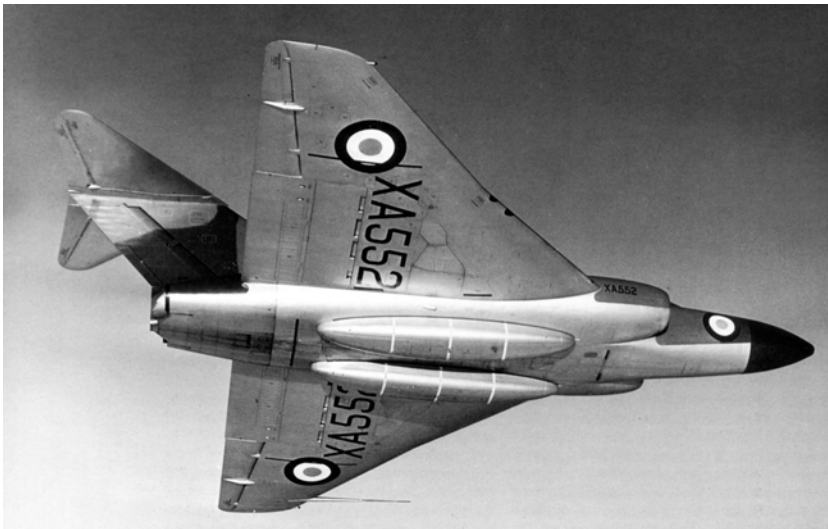
Early production Javelin with external fuel tanks, illustrating the restricted space available for carriage of an externally mounted bomb on a centreline station.
