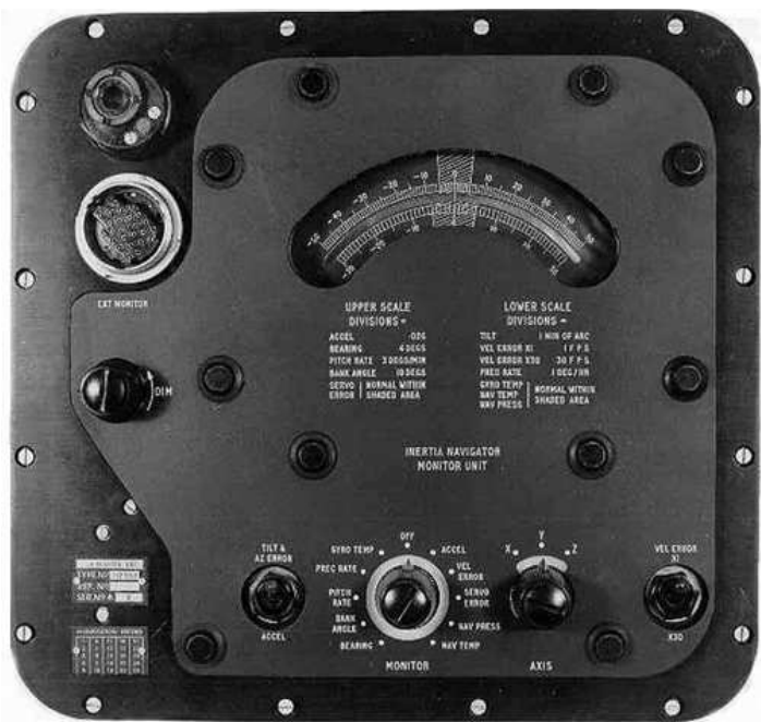
Above, the INCU, below, the INMU two, of the four units, which permitted the Nav Plotter to interface with the Missile.
