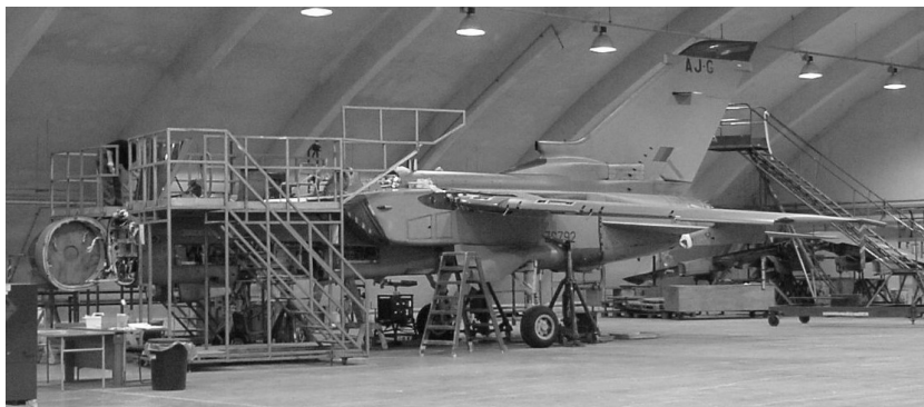
A Tornado undergoing a major overhaul at St Athan.
