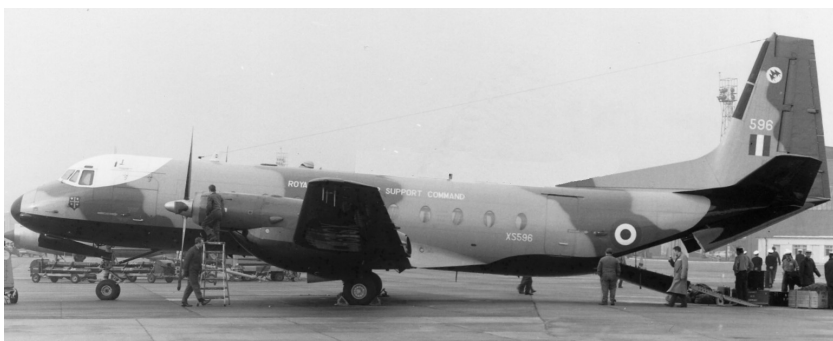
The Andover had a kneeling undercarriage in order to reduce the gradient of the access ramp.
