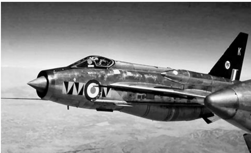
A 74 Sqn Lightning, XS897, in ferry configuration –refuelling probe under the port wing, OWTs and no missiles (this aeroplane was actually en route Singapore-Cyprus in 1971. (Dave Roome)
