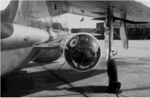
Left – head-on view of Red Top and its vulnerable hemispherical glass nose. Right – the Tigers’ aerobatic team.
