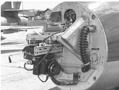
A local modification that installed a sideways-looking F95 camera in place of the gun ranging radar in two of No 20 Sqn's Hunters to provide a notional tactical recce capability.
