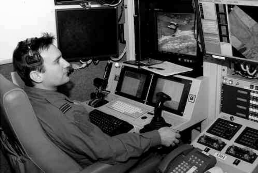
The pilot of a two-man RPAS 'crew' (the sensor operator has a similar console, out of shot to his right) at Creech AFB, Nevada controlling a Reaper flying – where? (MOD)
