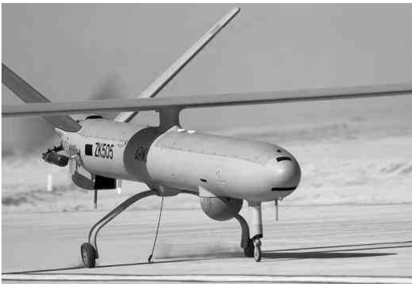
A leased Elbit Hermes 450 RPAS operated by the British Army pending deployment of the delayed Watchkeeper system. Both are unarmed passive systems and thus restricted to '3Ds tasks'. (Thales)
