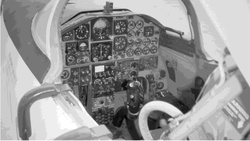
The front cockpit of a T-38A in the 1990s; the original analogue instrumentation has since been replaced in the re-fitted T-38C by digital displays incorporating a HUD, GPS and INS.
