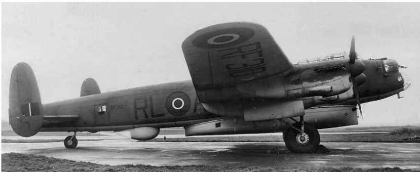
With a 31-foot Mk II airborne lifeboat fitted, RF310, was one of the first Lancaster ASR IIIs to be delivered to No 279 Sqn.
