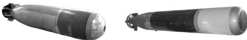
Left, an inert 18-inch Mk 30 torpedo and right, the much slimmer Mk 44. (RAF Museum)
