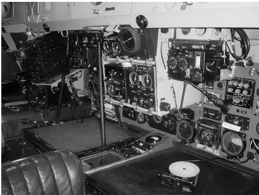
The navigators' station in a Mk 3 Phase 3 – Tac Nav on the right.
