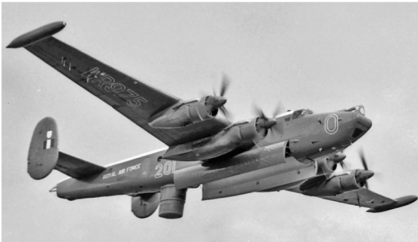
A Shackleton in the attack configuration – bomb doors open and radar ‘dustbin’ fully extended. (Jerry Hughes)
