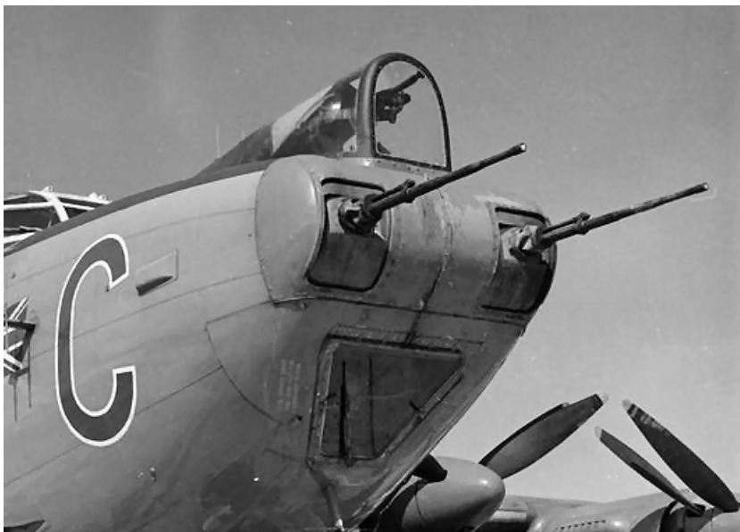
The Boulton Paul Type N gun mounting of a Mk 3 Shackleton.
