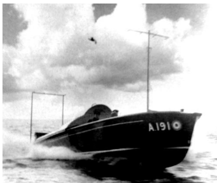
A191 – the second, of the seven, 37.5 ft armoured target boats. ( http://www.rafboats.co.uk )
