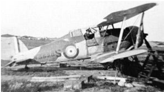
Above, N5520 (Times of Malta) and, below, N5519 (IWM) the latter fitted with the standard fixed-pitch Fairey-Reed propeller with a spinner.
