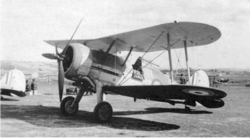
One of Malta's Gladiators, N5520, was fitted with a Mercury VIII engine taken from a Blenheim I, along with its variable-pitch, three-blade DH-Hamilton Standard propeller (IWM)
