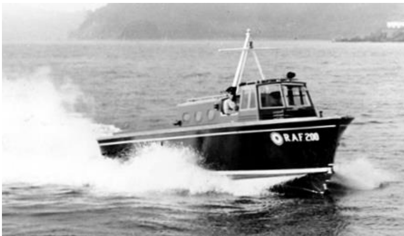
RAF 200 – the first of ninety-two 37·5 ft Seaplane Tender Mk Is. ( http://www.rafboats.co.uk )
