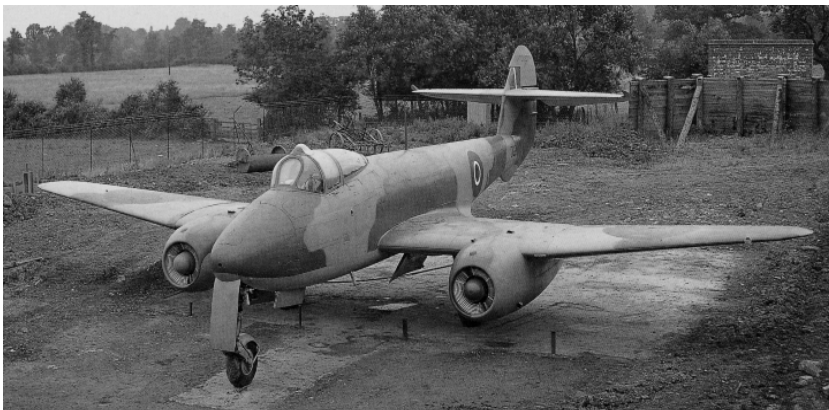
The Metrovick F.2-powered F.9/40 that was lost, along with its pilot, Sqn Ldr Davie, on 4 January 1944. Note that the axial F.2s were installed in Me 262-style underslung nacelles.
