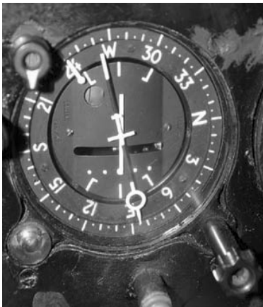
The Vulcan's Smiths Military Flight System was not as user-friendly as some.
