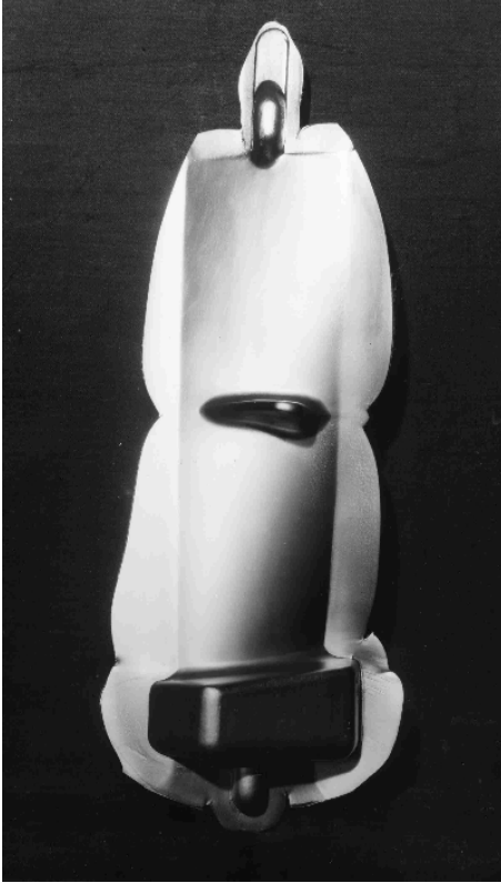
A titanium alloy compressor blade for an RB.199 engine. Forged-to-size, after the excess metal (flash) has been removed and the root block machined, it will be ready to fit. The pips at each end help with the machining operation. (HDA)
