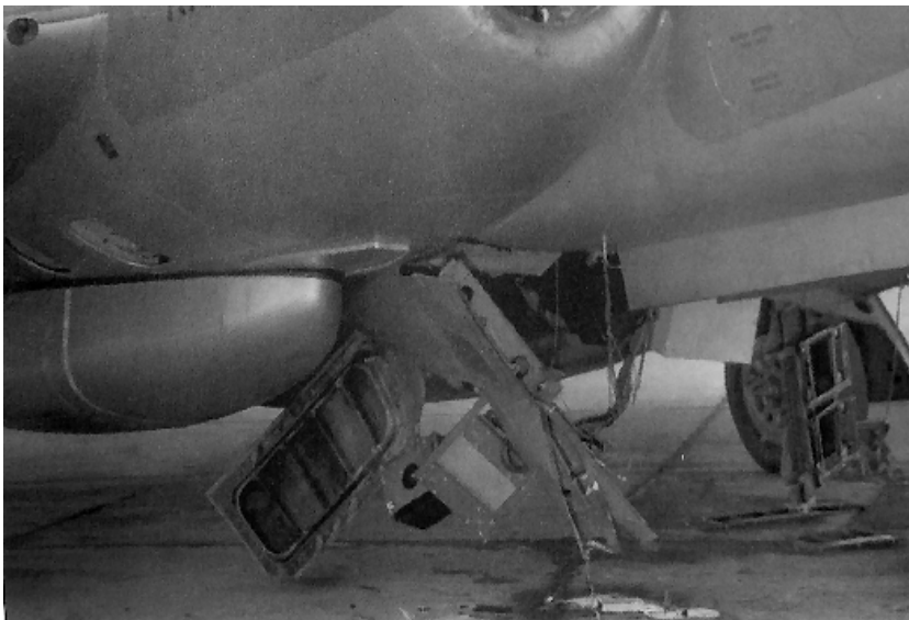
Cartridge starting 'could be explosive, as we found with the Sapphire starter on the Javelin.'
