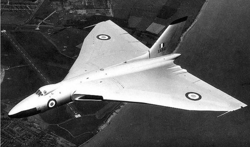
A Vulcan Mk 1 with the kinked Phase 2 wing.(BAE Systems)
