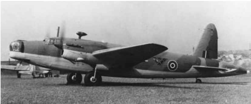
Above, one of the Hucknall-based Wellingtons used by Rolls-Royce to test jet engines, Below ,installation of a Whittle engine in the tail of a Wellington test-bed. (Rolls-Royce Heritage Trust)
