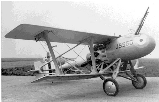
Sporting its massive 20mm cannon, Vickers rather outré response to Specification F.29/27 was a mid-engined pusher.
