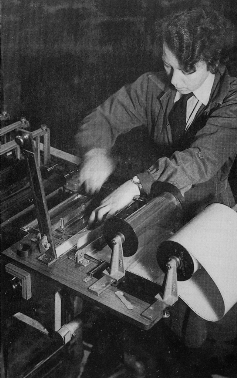
Continuous film developing machine – 1943
