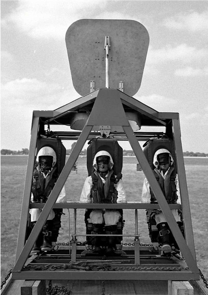
The rig built to demonstrate the feasibility of installing three rearward facing seats in a V-bomber.
