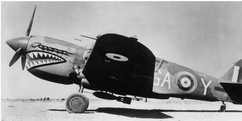
A Kittyhawk of No 112 Sqn at Gambut in mid-1942 armed with a 250 lb GP bomb fitted with an extension rod.(Andy Thomas)
