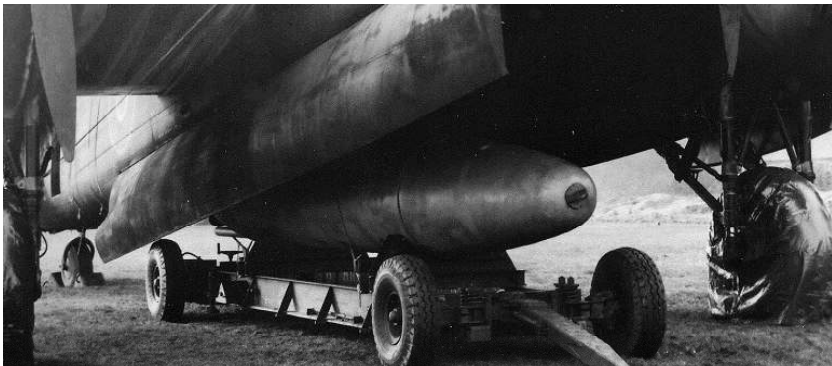
The prototype of the enormous Helmore Projector being loaded into a Lancaster in 1944.
