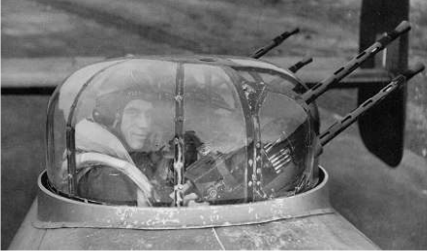
An example of a dorsal turret, the Boulton Paul Type A in a Halifax. Note the lack of space – a feature common to many turrets.
