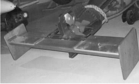
A MAT Mk III, fitted to a Mk XII torpedo, is on display at Hendon beneath the RAF Museum's Beaufort.
