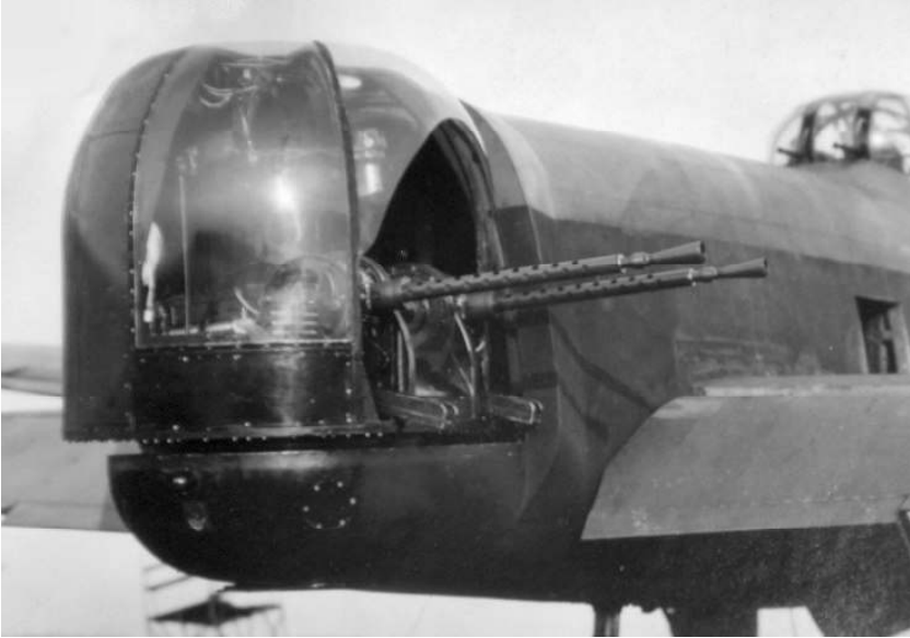
The roomy and uncluttered Rose turret with its large unglazed area and its twin 50-calibre guns set wide apart.
