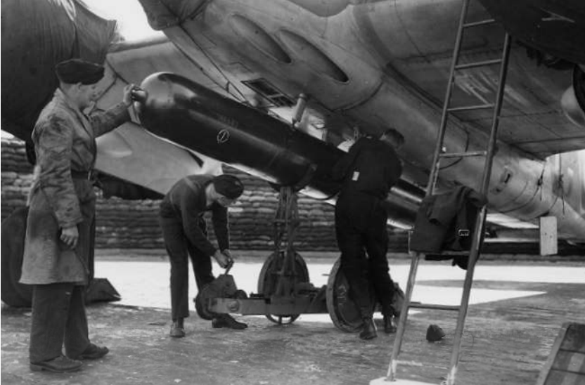
By 1944 the standard armament of the 'Torbeaus' of the UK-based Strike Wings was the Mk XV torpedo with a Torpex warhead, a Duplex pistol and a MAT Mk IV.
