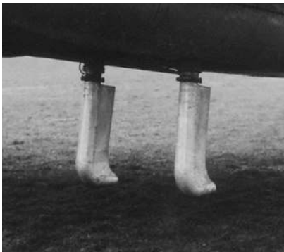
The ultimate design of streamlined discharge pipes, seen here on a Blenheim.
