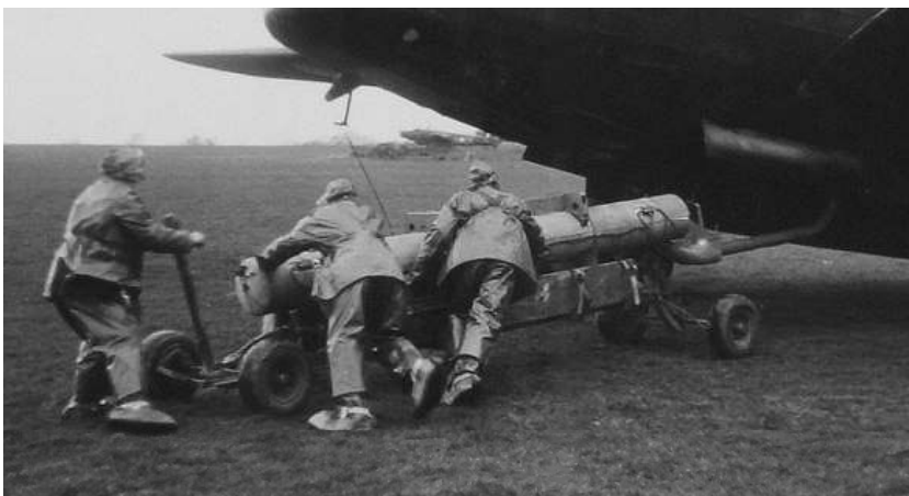
Armourers in full protective clothing manhandling a 1,000 lb SCI towards the bomb bay of a Wellington during a trial carried out at Feltwell in 1941. Note the long extended and articulated discharge pipe.
