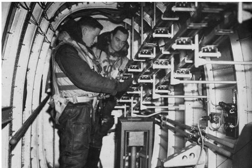
Air gunners checking the ducts, or tracks, which fed ammunition from the mid-fuselage magazines to the four-gun turret in the tail of, in this case, a Halifax but the arrangements were much the same in both the Stirling and the Lancaster.
