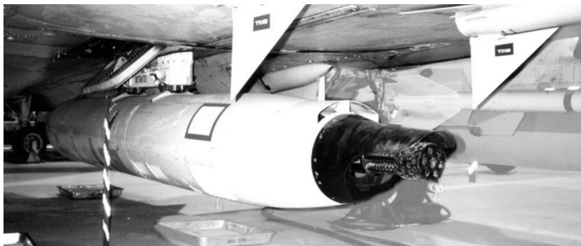
The American 20mm M61 rotary cannon which saw service with the RAF in the form of the Phantom's SUU-23 gunpod.
