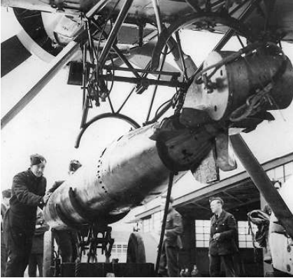
A Mk VIII torpedo fitted with a drum-type drogue on a Vildebeest.
