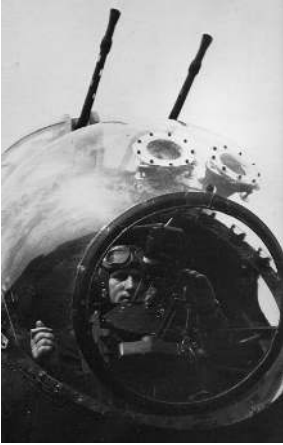
The infrared 'headlights' of the 'Z' IFF installation.
