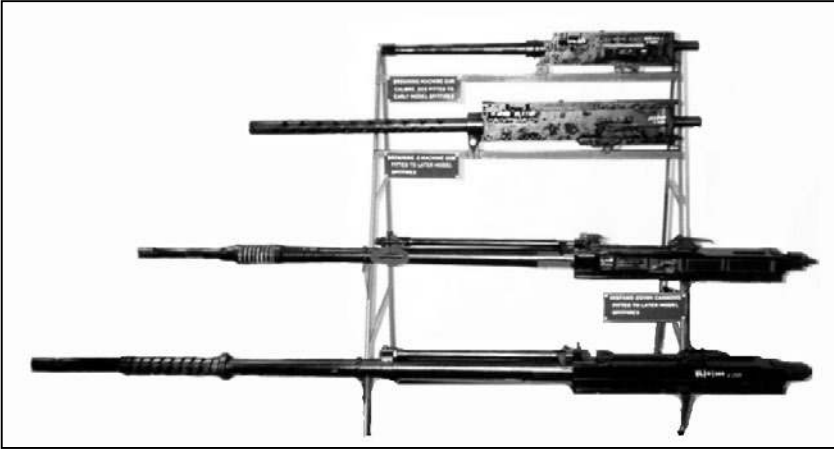
Comparative sizes of wartime RAF guns. From the top: the .303" Browning; the .50" Browning; the short-barrelled Hispano Mk V and the standard Mk II.
