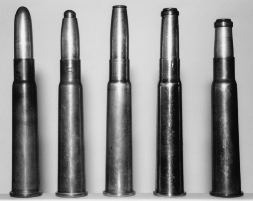
Examples of .303" aircraft gun ammunition: PSA (Pomeroy) Mk I (HE); PSA Mk II; RTS Mk II (HEI); RTT (experimental HEI); and R Mk III (experimental HE).
