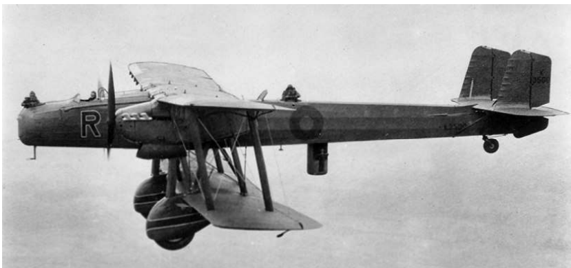
The Handley Page Heyford with its retractable ventral 'dustbin' in the extended position.
