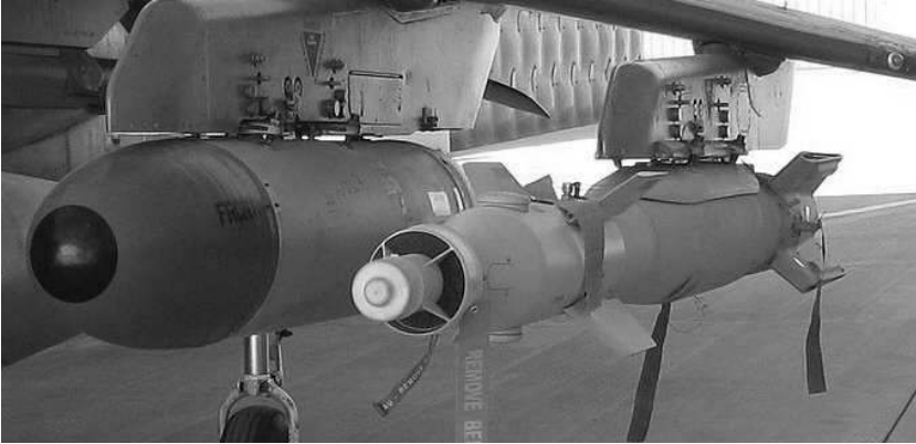
A 500 lb Paveway IV and CRV-7 pod, complete with nosecone. (MOD)
