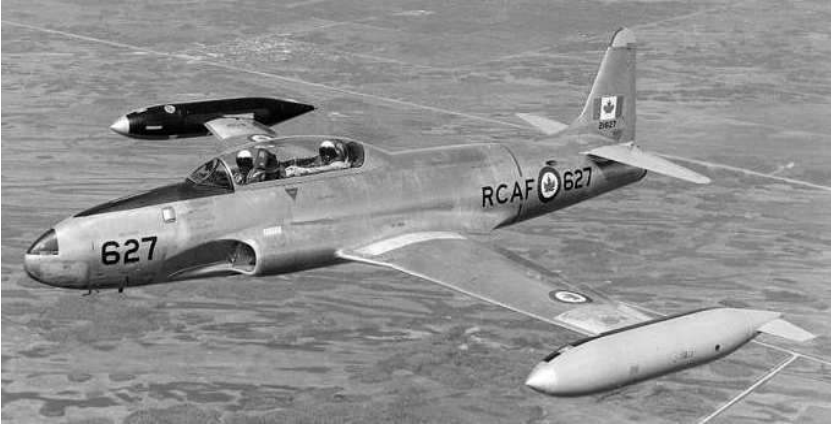
The Nene-engined, Canadair-built CT-133 as used by the NATO Air Training Plan in the mid-1950s.
