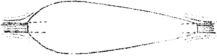
Fig 8. Sketch from Whittle's 1931 paper showing how a jet engine facilitates a clean, minimal drag installation.
