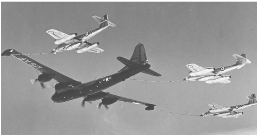
The three-point YKB-29T, modified by FRL for Project OUTING, refuelling two Meteor F8s of No 245 Sqn and FRL's Meteor IV VZ389. (FRL)
