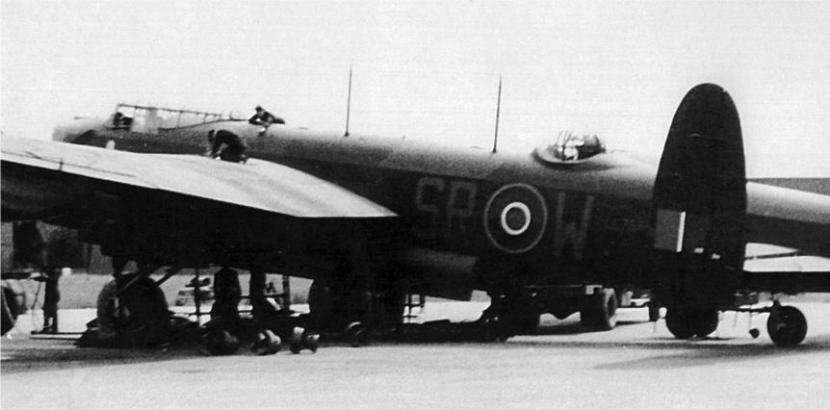
A Lancaster of No 101 Sqn with the mast aerials of Airborne Cigar ahead of the dorsal turret.
