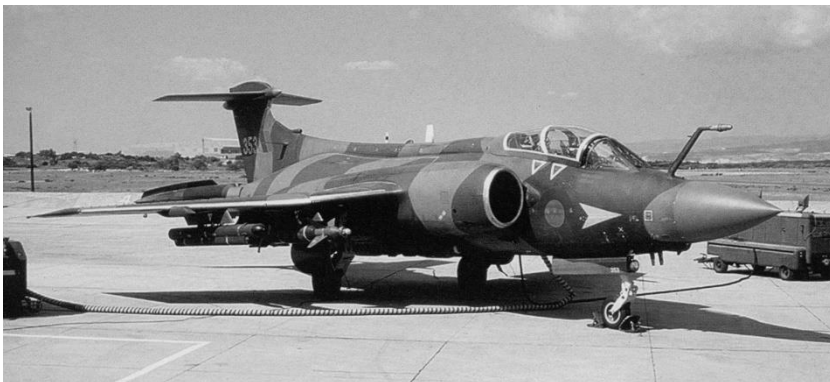
One of the Op PULSATOR Buccaneers at readiness with an LGB and an ALQ-101 ECM pod visible under the starboard wing. (G Pitchfork)
