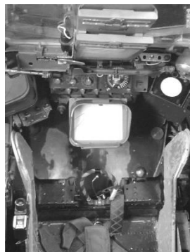
Left, the Pavespikes pod and, right, the Paveway display located between the nav's knees.
