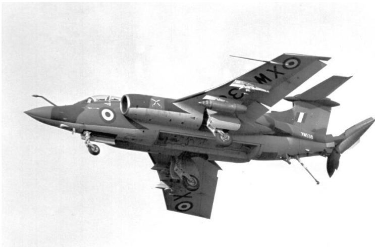
A Buccaneer S2B, XW538, of No 237 OCU letting everything hang out – undercarriage, arrestor hook and flaps down, ailerons drooped, air brake open, bomb bay rotated open – and a single SNEB pod on the port inner pylon. (MAP)
