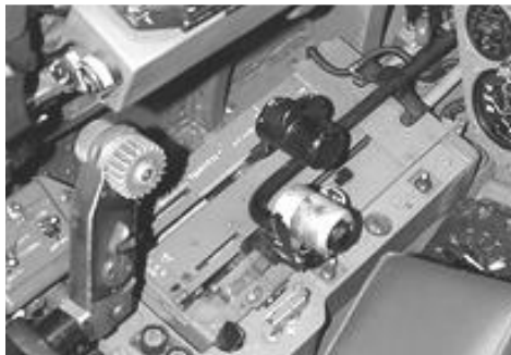
Left, the AI 23 controller and , right, its location aft of the throttle box. ( www.firestreakbooks.com )
