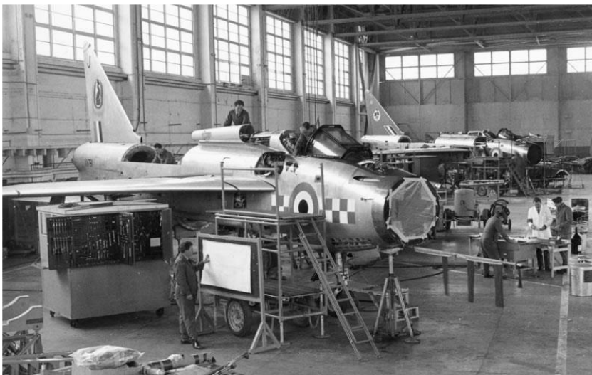
Lightnings, in this case of Nos 19 and 92 Sqns, undergoing second line servicing.
